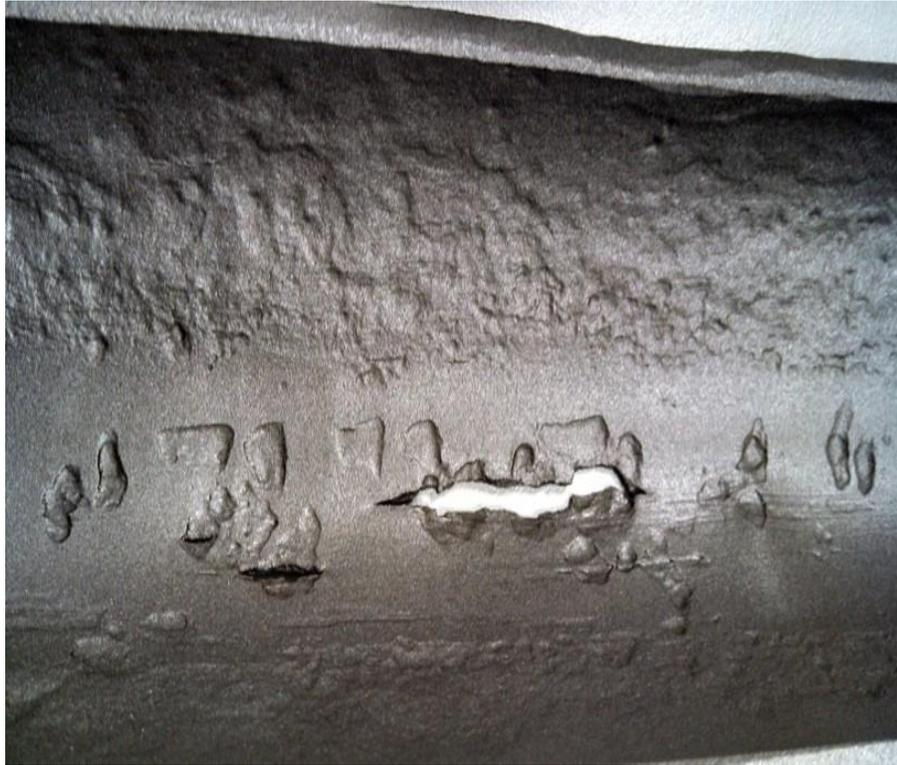
**Figure 1: Pitting on a steel pipe due to microbiologically influenced corrosion.**
