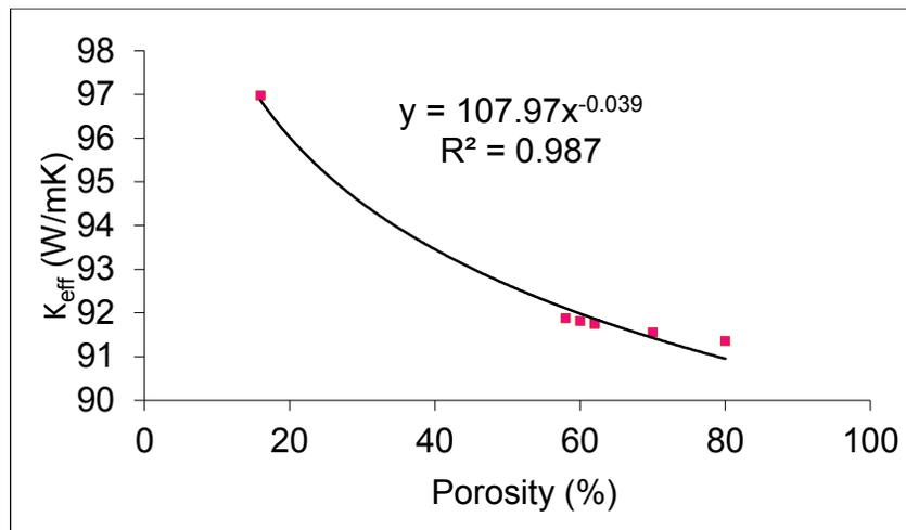
**Figure 6: Effective thermal conductivity as a function of porosity (%).**
