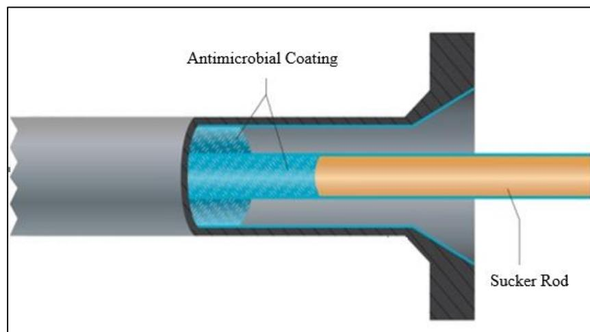
**Figure 2: Antimicrobial coated well schematic.**
